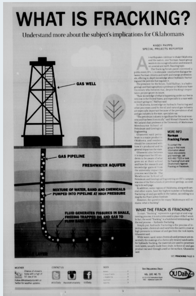
Fig. 16.13: This graphic from OU's student newspaper The Oklahoma Daily shows how fracking works. First, a mixture of water, sand, and chemicals is injected into the ground at extraordinarily high pressure. This process creates cracks deep underground, which free oil and gas trapped in a layer of shale, allowing the oil and gas to be extracted for production.
